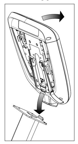
Figure 15: Console positioning on base unit
