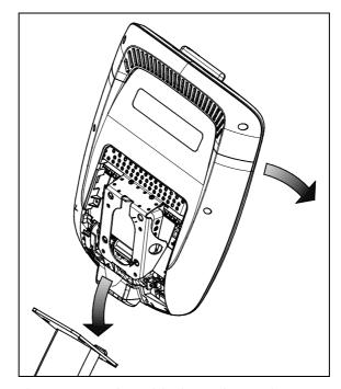
Figure 9: Console positioning on base unit
