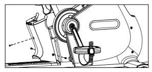
Figure 4: Rear cover removal
