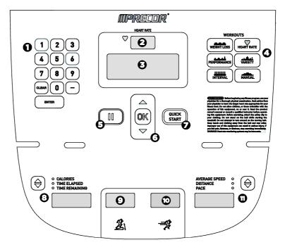
Figure 4: P10 console keys
