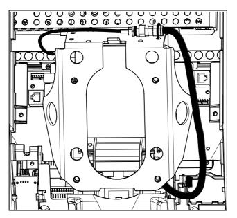
Figure 11: Connecting the television cable
