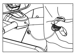
Figure 7: Attaching the safety clip
