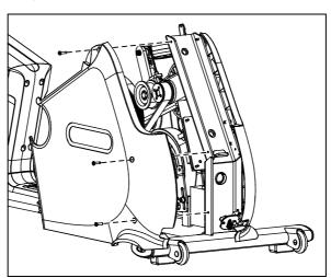
Figure 5: Left side cover removal
