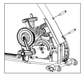
Figure 7: Bolting the upright support into place
