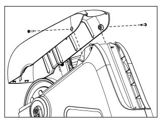
Figure 3: Top cover removal
