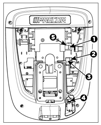
Figure 18: Cable connections, P30 and P10 consoles
