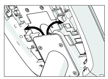
Figure 17: Cable routing from the mount into the console
