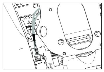
Figure 13: Connecting the heart rate cable
