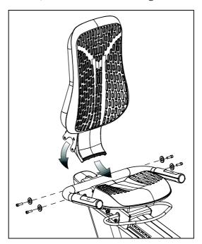
Figure 2: Moving the seat back assembly into position
